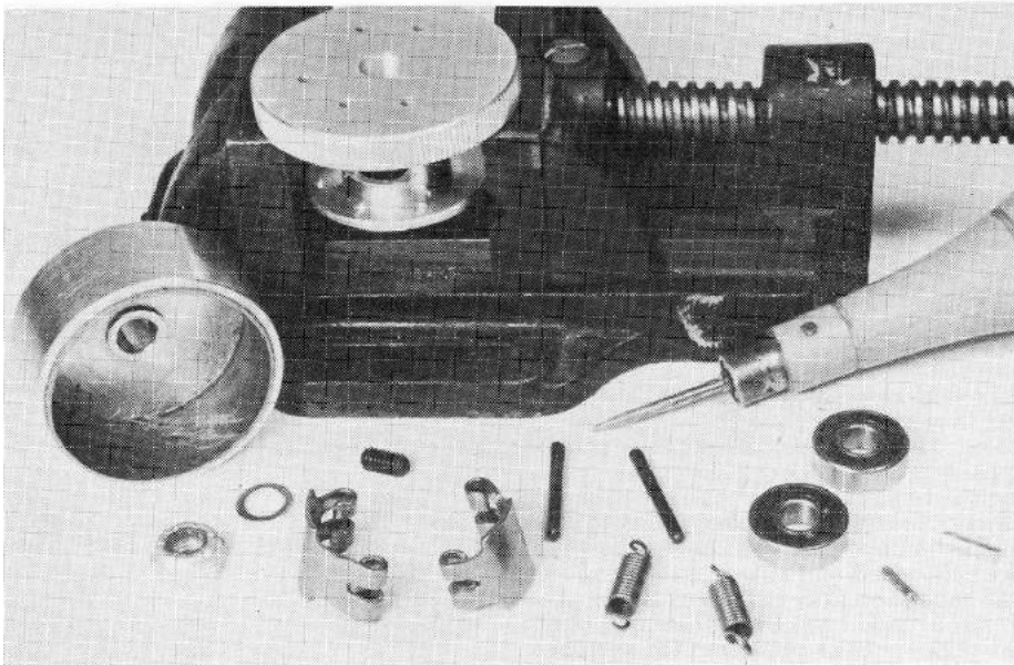
Parts for the clutch laid out with machine vice for fitting.
